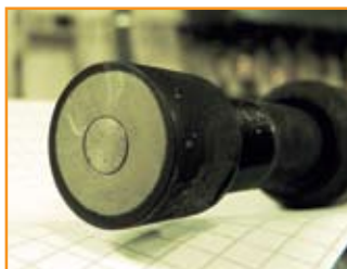
Ultrasound keeps the active surface of the OptoSono probe clean.
